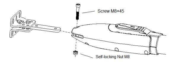
**E)** As shown in figure 8 below, connect wall bracket with wall according to marked position. Then, connect main machine with wall bracket by screw and nut. (Please use spirit level to make sure the installation levelness.)
