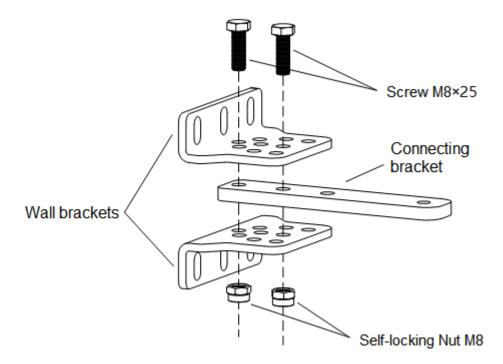
B) The connecting bracket and the wall bracket can be connected according to different conditions, please refer to figure 5.
